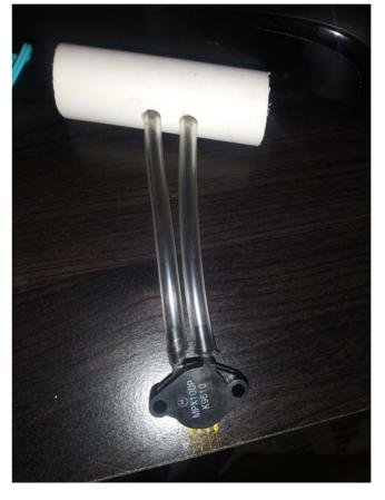
Differential Pressure Pneumotachometer Circuit (Winter Qtr.)
