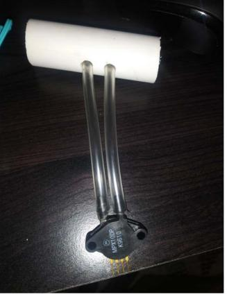
Differential Pressure Pneumotachometer Circuit (Winter Qtr.) Differential Pressure Pneumotachometer Circuit (Spring Qtr.) LabView Data Acquisition Unit "Airway adapter" and sensor for pressure/flow rate
