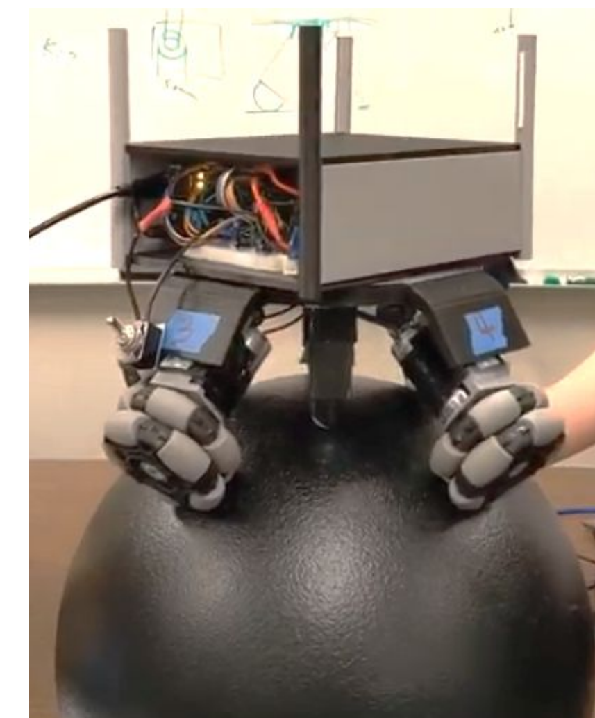
Fig. 9. The final deliverable of the ball-balancing robot (Picture credit: the Piqard team)
